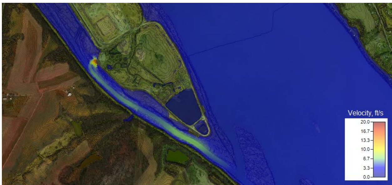
Figure 3.3-3 HEC-RAS 2D Dam Failure Simulation – Northwest IDF Breach Scenario
